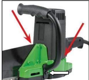
The auxiliary handle can be mounted on the left or on the right side of the machine, depending on the operation method.
